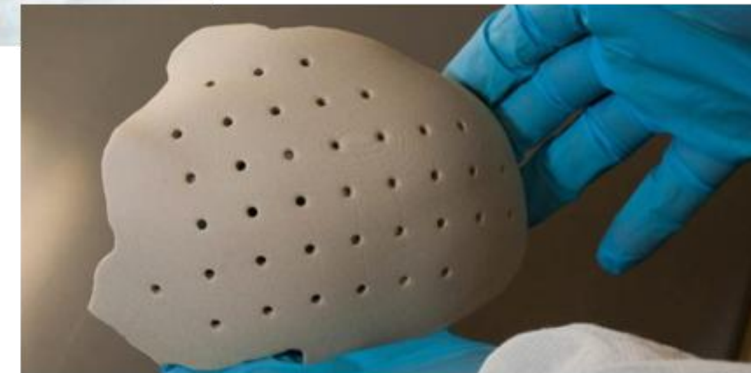
An OXPEKK SLS 3D printed cranial implant [Image credit: Oxford Performance Materials]
